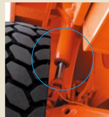
The ACCU-TRAC suspension design allows the front struts to be removed and installed without removing the trailing arms, brakes or tires. This relates to fewer tools and less labour required to perform the repair, which aims to reduce the amount of hauler downtime, increasing productivity.
